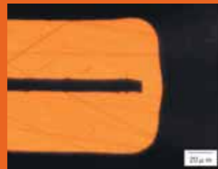
CROSS SECTIONAL AFTER PLATED — FARADFLEX® BC12
